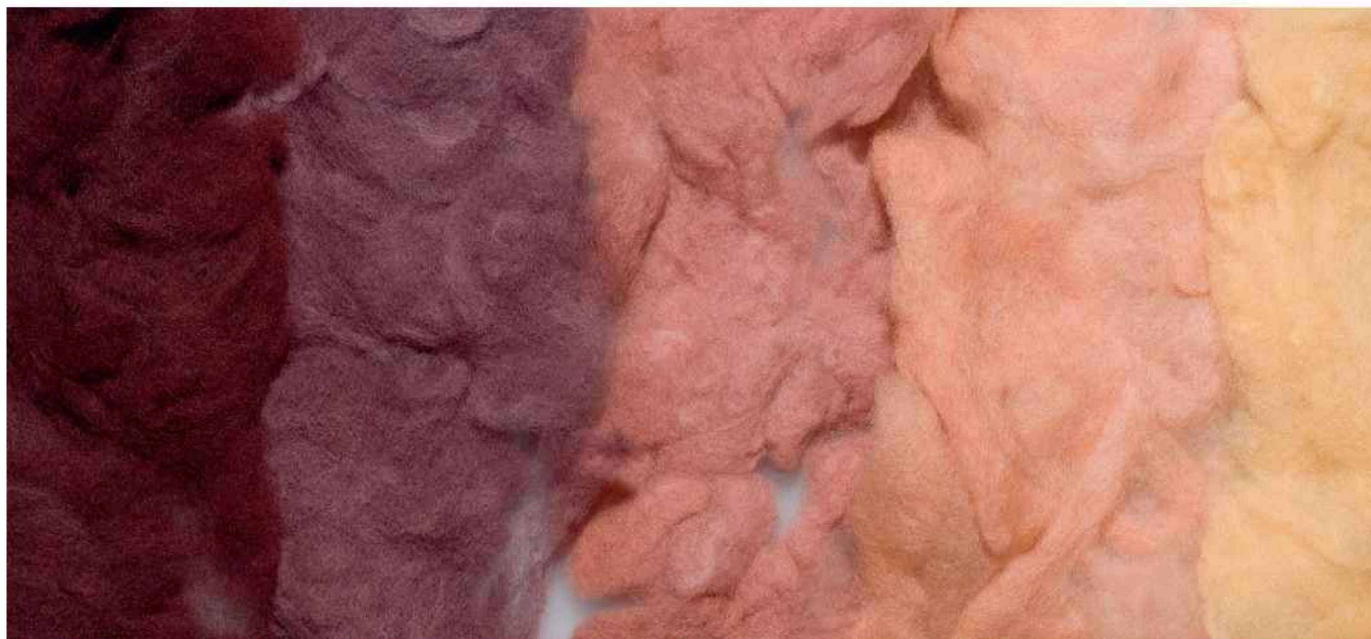
New Zealand Merino wool coloured with silver nanoparticles. Picture from Robert Cross, Images Services, Victoria University of Wellington.
