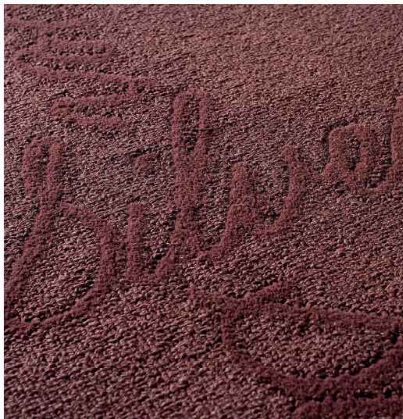
A carpet sample made by the UK-based Wools of New Zealand, from New Zealand wool coloured with silver nanoparticles. It is also anti-microbial and anti-static. Picture from Robert Cross, Images Services, Victoria University of Wellington.
