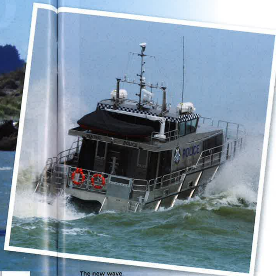
The new wave piercer design aids in sea keeping ability
