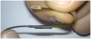
Figure 1. The flexible Hall probe K
