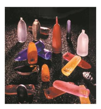
From scratch, the sapphire is with his purity of 99.99% transparently colorless. His different colors are given with the addition of metal oxides. In the case of a ruby it is chromium, in the case of a blue sapphire it is titan and iron, to a purple sapphire it is vanadium, and to a yellow or green one it is iron, which is added.
