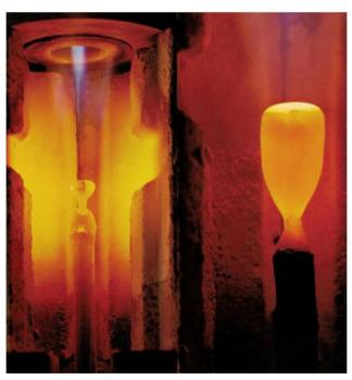
The annealed powder is put bit by bit and in small portions into the Verneuil burner, where it drops through a cylinder with the influx of oxyhydrogen. What takes millions of years to be built by nature is, because of the very high temperatures, formed within 212 hours: a pear shaped corundum crystal.
