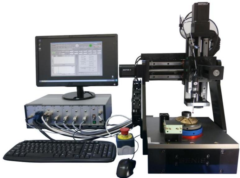
The SENIS Magnetic Field Mapper, or MMS-1A-RS, is a high-end magnetic field scanner that can be applied for mapping of all three components of DC or AC magnetic field. It can be used as a quality assessment tool in production lines for accurate 3D mapping of permanent magnets.
