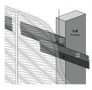
Fixing Distances: Panels should be fixed at least 1200mm.
