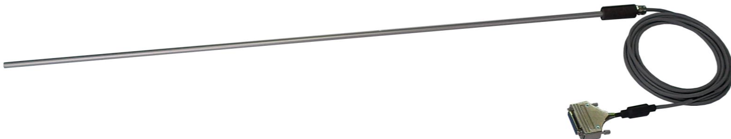
Figure 1. Photo of the PHS-C Probe Holder with a SENIS Hall probe installed enclosed in the holder
