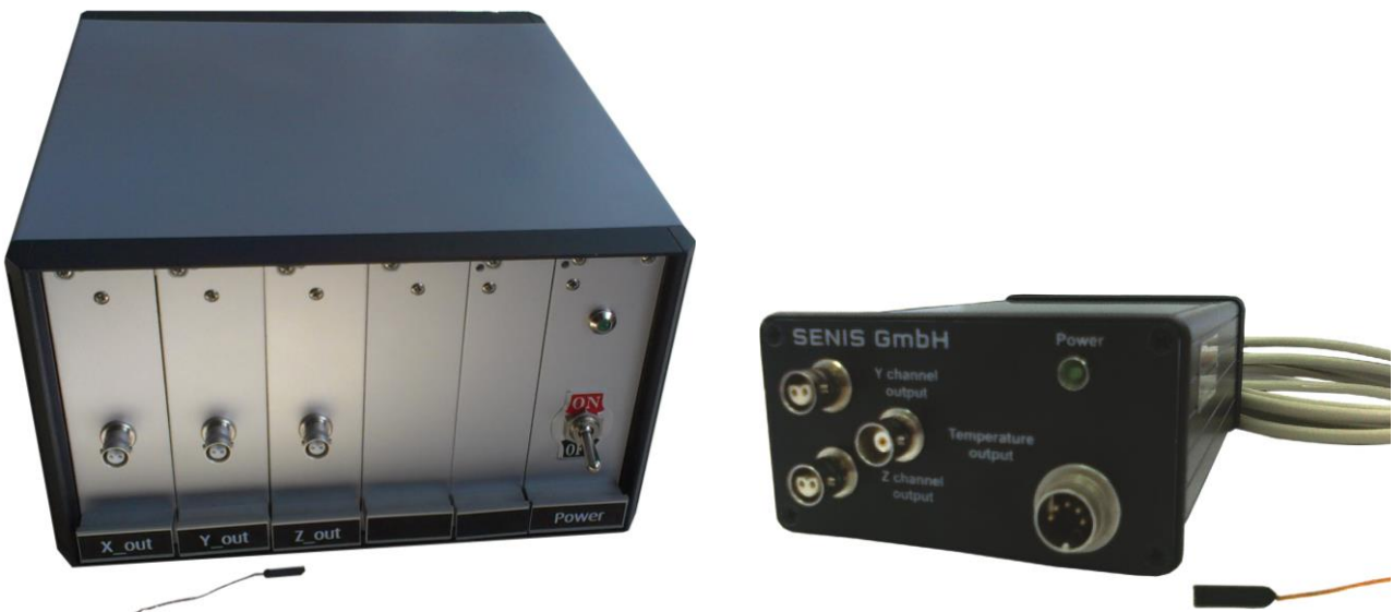
Figure 3. Photo of a 3-axis (box type G, left) and a of 1- or 2-axis (box type B, right) magnetic field transducer with hybrid Hall Probe
