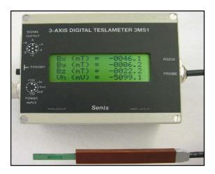
Fig. 5: SENIS magnetic measurement instrument (reprinted from Senis promotion material, 2004)
