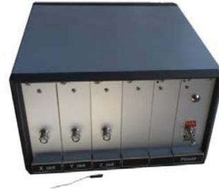
Fig. 6. SENIS Low-Noise magnetic field-to-analogue-voltage Transducer[4].
