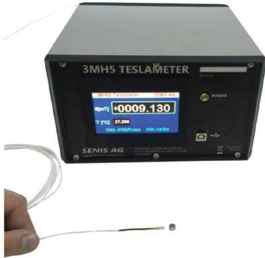
Fig. 8. SENIS High-Accuracy Teslameter with a very thin three-axis Hall Probe encapsulated in ceramic package
