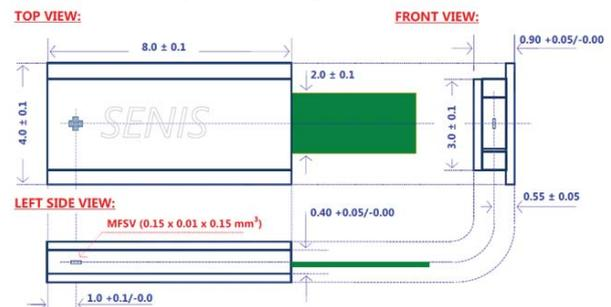
Fig. 4b. The dimensions of standard ceramic package of SENIS three-axis Hall probes (length x width x thickness): 8.0mm x 4mm x 0.9mm.
