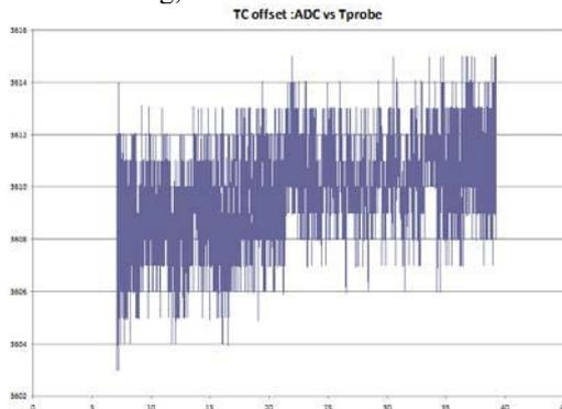
Fig. 9. The graph shows the AD-converter (ADC) reading during the Hall probe temperature change in the range of 30°C. The change is 6LSB (least significant bits), which corresponds to the temperature coefficient (TC) related to the Hall probe temperature of 0.1µV/°C. The TC related to the electronic module of Teslameter is 0.5µV/°C.
