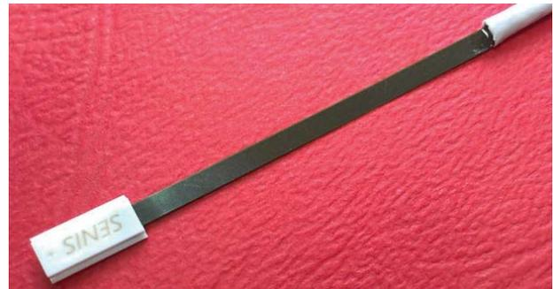
Fig. 4a. Photograph of the standard ceramic package of SENIS three-axis Hall probes. This package is suitable for the temperature range -55 $^{\circ}\text{C}$  to +155 $^{\circ}\text{C}$ .
