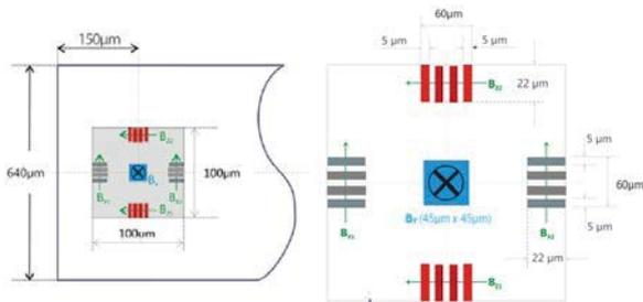
Fig. 2. The spatial distribution of the Hall devices of Fig. 1 on the Hall probe chip. The novel SENIS integrated Hall probes have the magnetic field sensitive volume) of 100 $\mu\text{m}$  x 10 $\mu\text{m}$  x 100 $\mu\text{m}$  ( $B_y$ : 45 $\mu\text{m}$  x 5 $\mu\text{m}$  x 45 $\mu\text{m}$ ;  $B_x$  and  $B_z$ : 100 $\mu\text{m}$  x 10 $\mu\text{m}$  x 100 $\mu\text{m}$ ).
