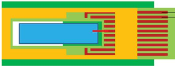
Fig. 5b. Structure of the ultra-thin SENIS ceramic package for three-axis Hall probes: the bottom and the cover plate are  $40\mu\text{m}$  thin machinable ceramic plates. The substrate is a  $100\mu\text{m}$  flex-PCB. The sensor IC die is Si CMOS IC,  $50\mu\text{m}$  thin, with  $20\mu\text{m}$  bonding wire loops.
