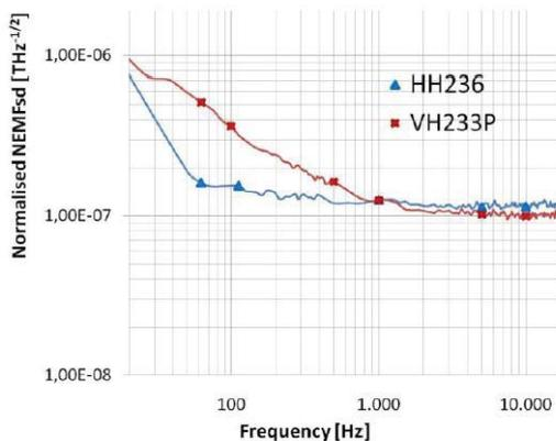
Fig. 3. Measured noise-equivalent magnetic field spectral density of the SENIS' Hall devices [4] implemented in 0.35 $\mu\text{m}$  CMOS technology, normalized to biasing power of 1mW. HH236: horizontal Hall device
