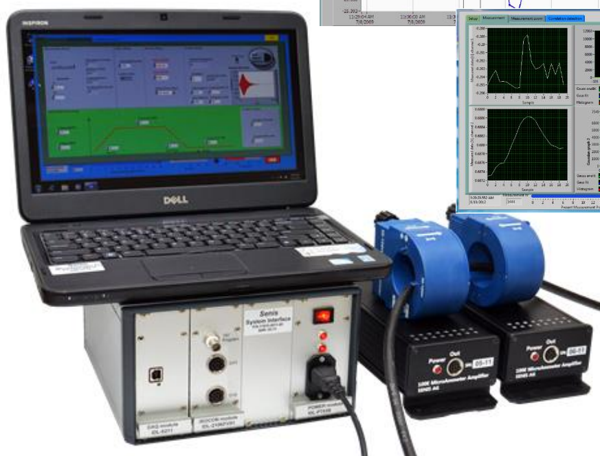
Figure 1. Insulation Defect Locator Measurements Setup
