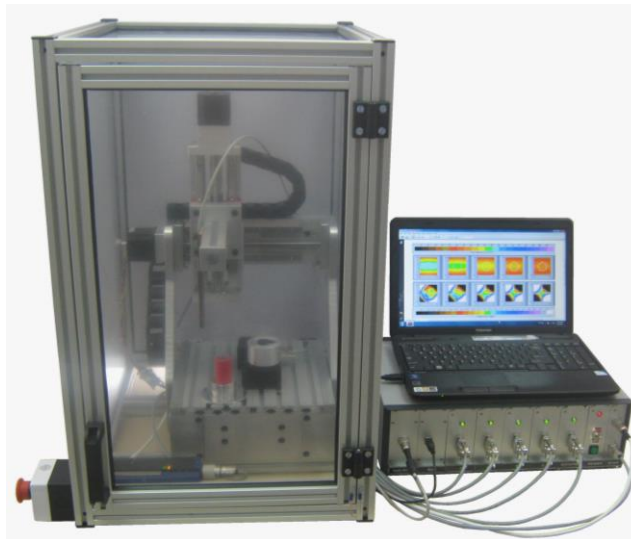
Figure 3: Scanning system MMS-1-RS equipped with the protection cabinet to satisfy the CE directives (mandatory for the production environments)
