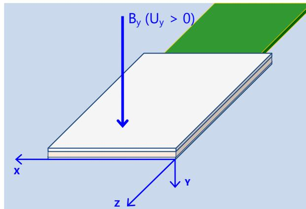
Figure 3. Reference Cartesian coordinate system of the integrated 0YU Hall probe
