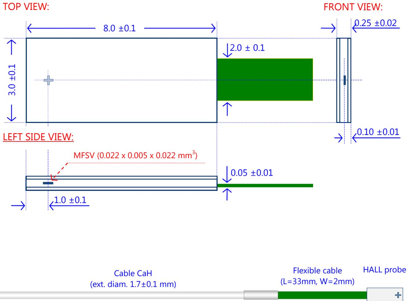
Figure 2. Dimensions and tolerances of the integrated 0YU Hall probe and cable CaH (Module H)
