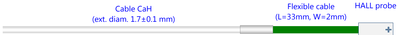
Figure 2. Dimensions and tolerances of the fully integrated 0YU Hall probe and cable CaH (Module H)
