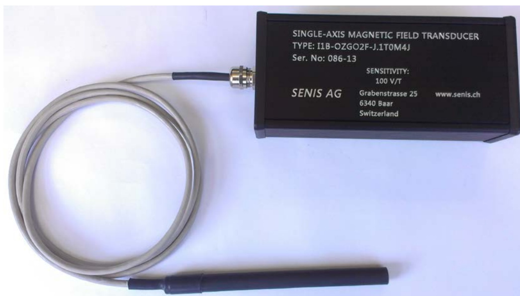
Figure 2. Single-axis analog magnetic field transducer type I1B-0ZG02F-J.1T0M4J
