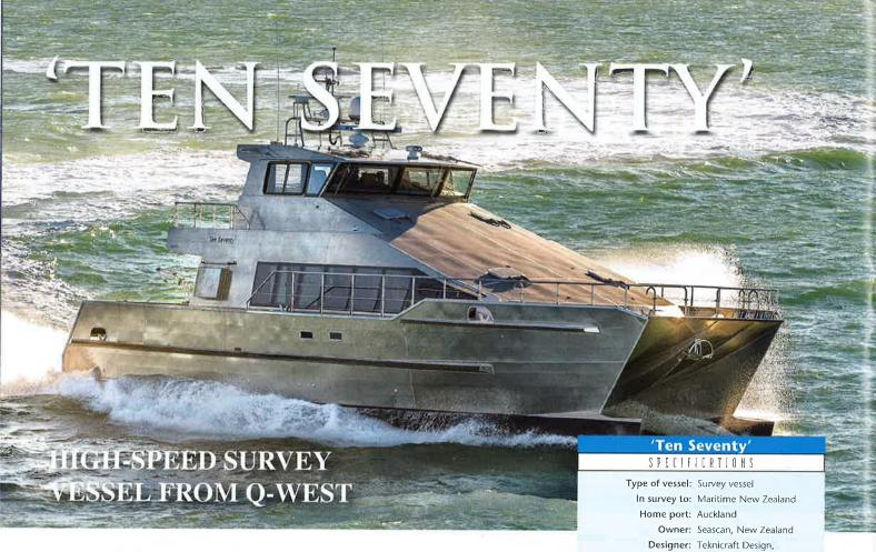
New Zealand naval architecture firm Teknicraft has incorporated a number of new design elements in 'Ten Seventy', a new foil-assisted survey catamaran which was built in New Zealand by Q-West Boat Builders.
