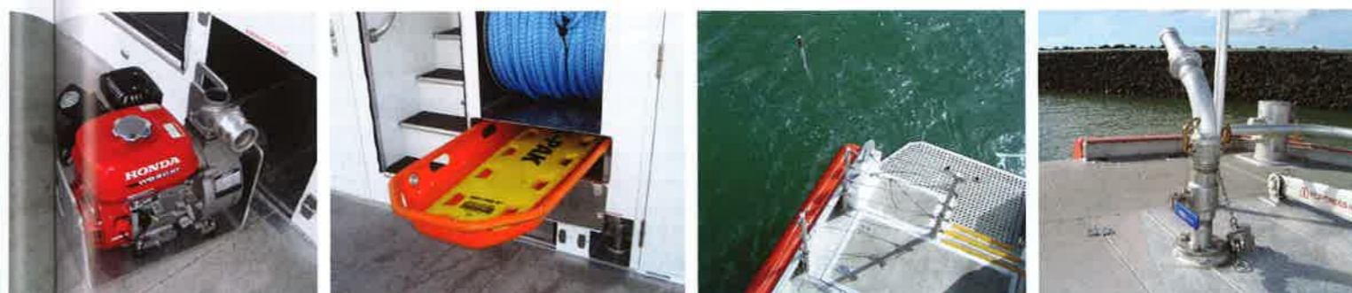
Honda portable pump Scoop and boat stretchers MOB stick Forward fixed fire nozzle
