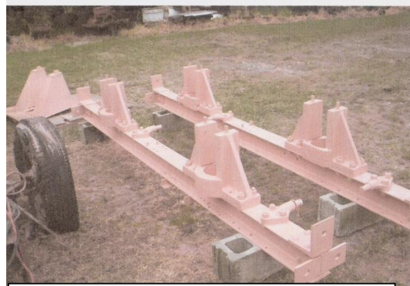
Chassis rails sandblasted and primed
