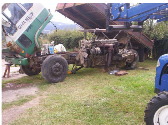
Removing the Isuzu motor from the truck donated by Mercers
