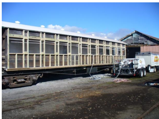
2 nd Side of carriage showing the new framing installed
