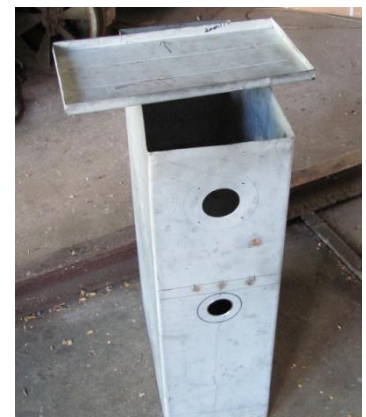
Fuel tank before painting
