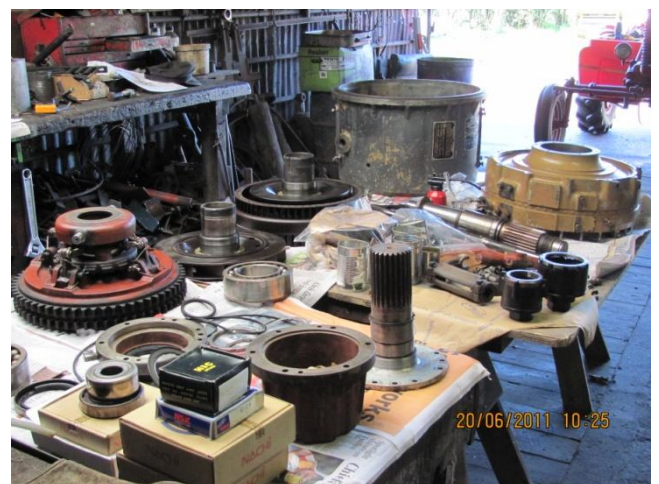
Torque Converter parts ready for assembly
