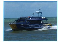
The vessel has a fuel capacity of 2,000 litres and consumes 5.9 litres per nautical mile, giving the vessel a range of over 300 nautical miles.
