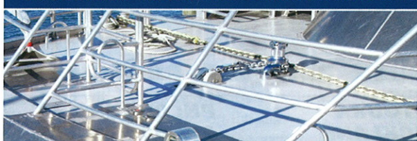
MAXWELL'S VWC4000 AND DEVILS CLAW INSTALLED ON 'MARAROJA', 19M ALLOY CATAMARAN, MANUFACTURED BY Q-WEST BOATS FOR MERIDIAN ENERGY.
