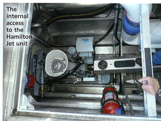
Easy access to the strum box and fuel filters aids servicing
