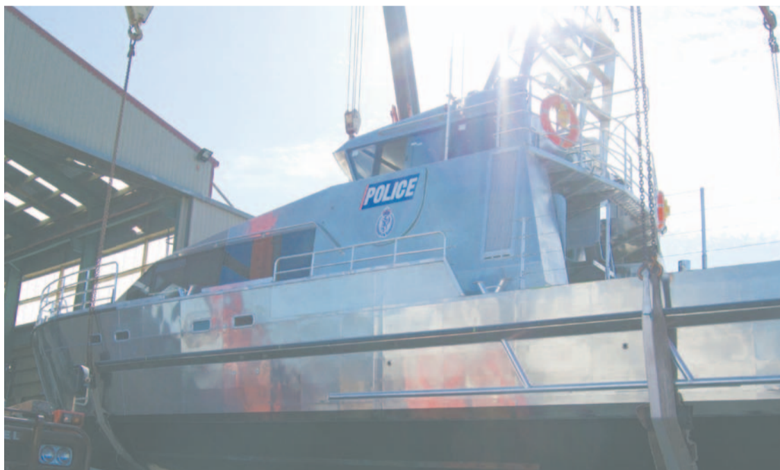
The 18.5m, twin-hulled aluminium vessel, Deodar III, has been built by Q-West Boat Builders for the New Zealand Police
